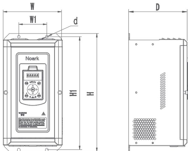
图2-8-2 Ex9VF3-0110CT43 ~ Ex9VF3-0220VT43外形和安装尺寸图
