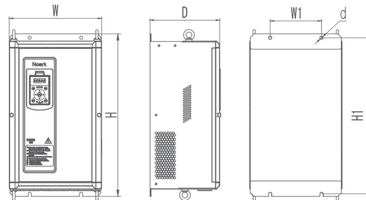
图2-8-3 Ex9VF3-0220CT43 ~ Ex9VF3-0750VT43外形和安装尺寸图
